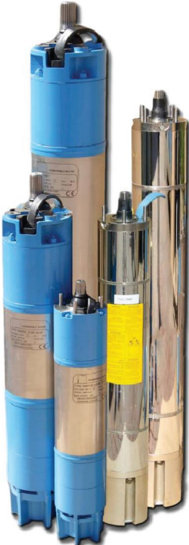
Series of submersible motors 6 "rewindable water bath, asynchronous 2 poles, with squirrel-cage rotor. Winding wire wet PVC, easily retractable. Durable engines oversized to withstand heavy loads and long life. The radial and axial Bearing are Mitchell and lubricated by water inside the motor; this allows a long period of operation without any maintenance. Mechanical Seal mounted sull'Driving shaft which allows a particular strength in the presence of sand.
